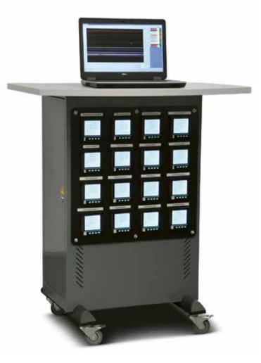
This measuring device has been developed in cooperation with ETH Zurich / Inspire. Up to 16 electrical channels and one air pressure channel can be evaluated. Recording is automatic and results in a diagram like the one shown above.
